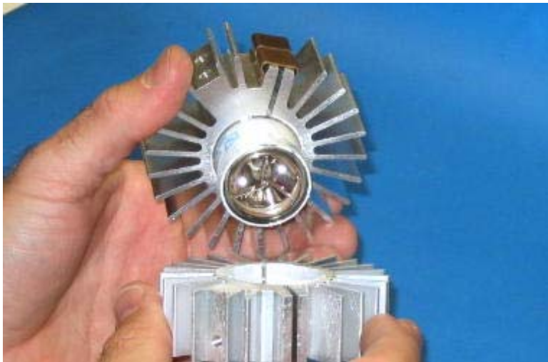
Step 5: Cathode heatsink being removed. If the cooling ring which mounts around the window stays attached to the lamp, remove it and set aside. You may choose to leave the cooling ring in the cathode heatsink, but must assure that the new lamp is fully seated when installed.
