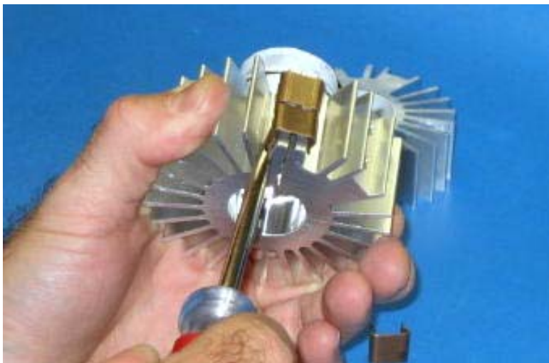
Step 6: Spring clips being removed from anode heat sink.
