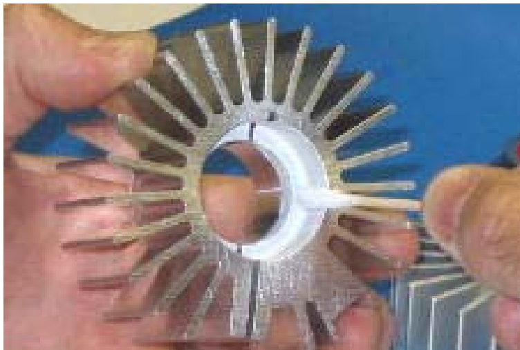
Step 8: Apply thermal compound to anode heatsink. The anode heatsink is 1.25" thick and has a 1" through hole to accept the lamp base. There are three areas that will mate with the lamp. Assure all three are coated with compound.
